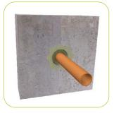
Cut nozzle to required bead size and apply sealant around the service and fill the void to the surface of the substrate using an appropriate caulking gun. Best results are achieved if filling is started at the bottom of the void and working upwards.
