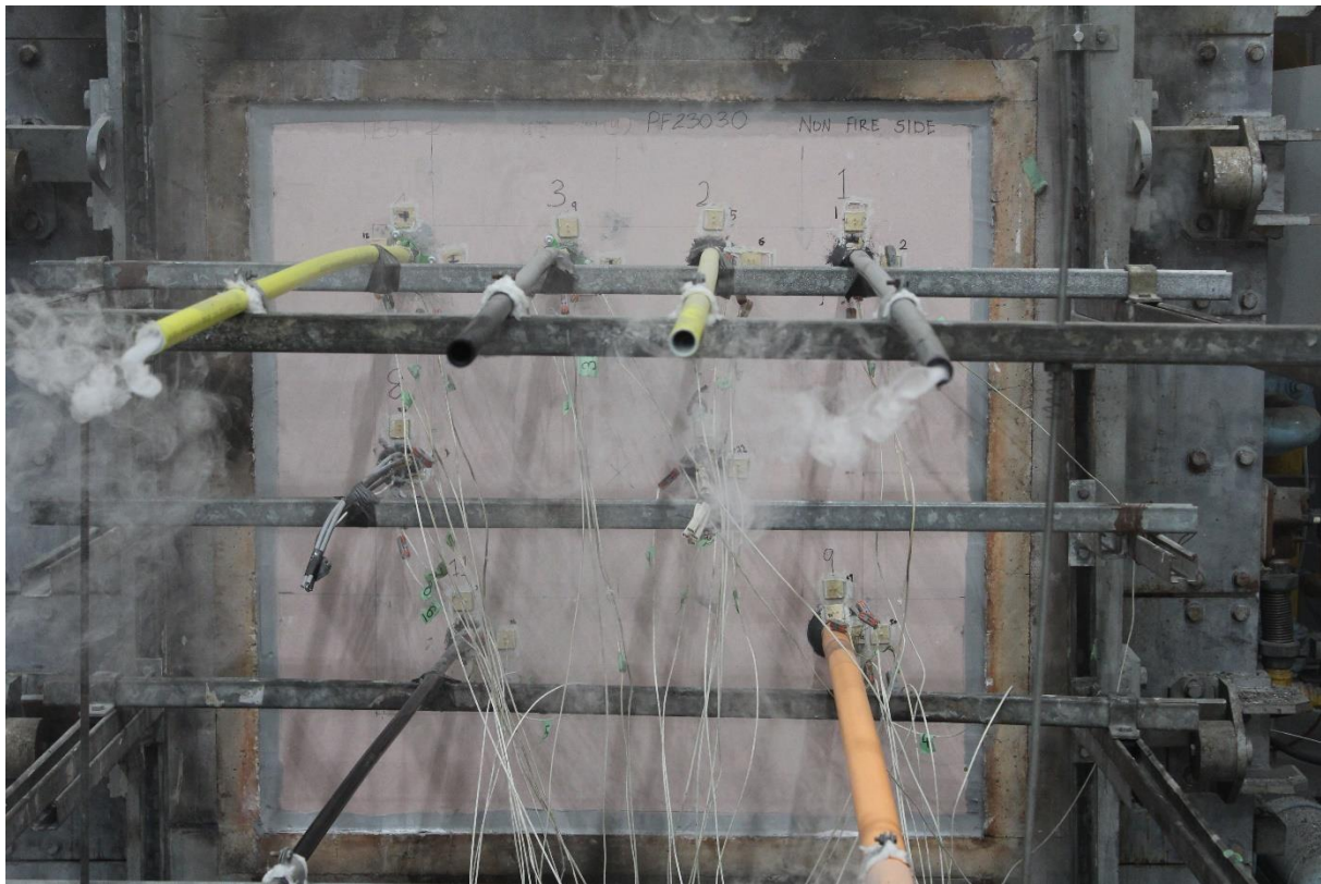
Figure 35 – Unexposed face at 30 minutes
