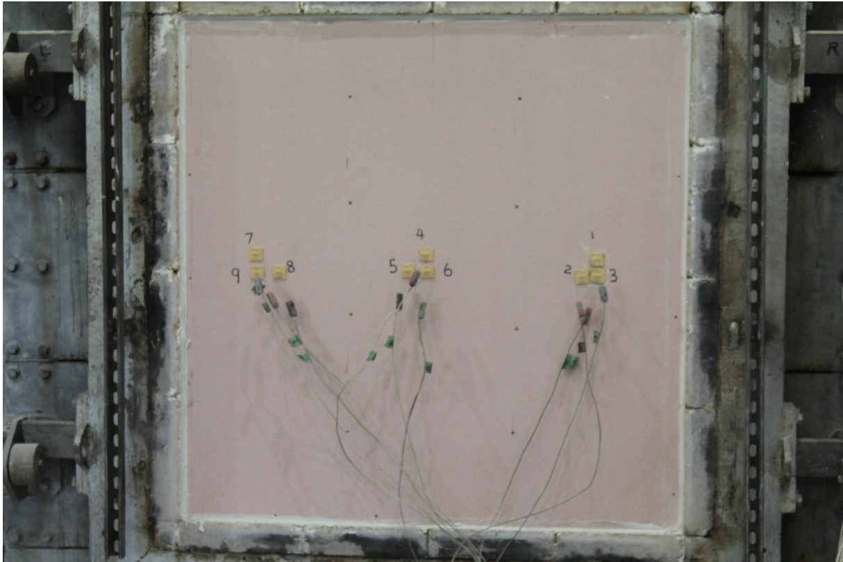
Figure 47 – Unexposed face at 60 minutes
