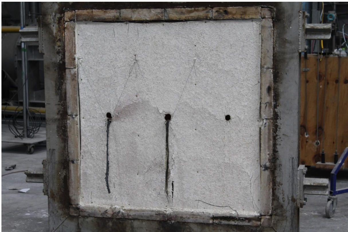
Figure 50 – Exposed face after the test
