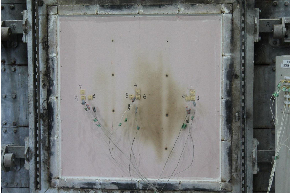
Figure 49 – Unexposed face at 90 minutes
