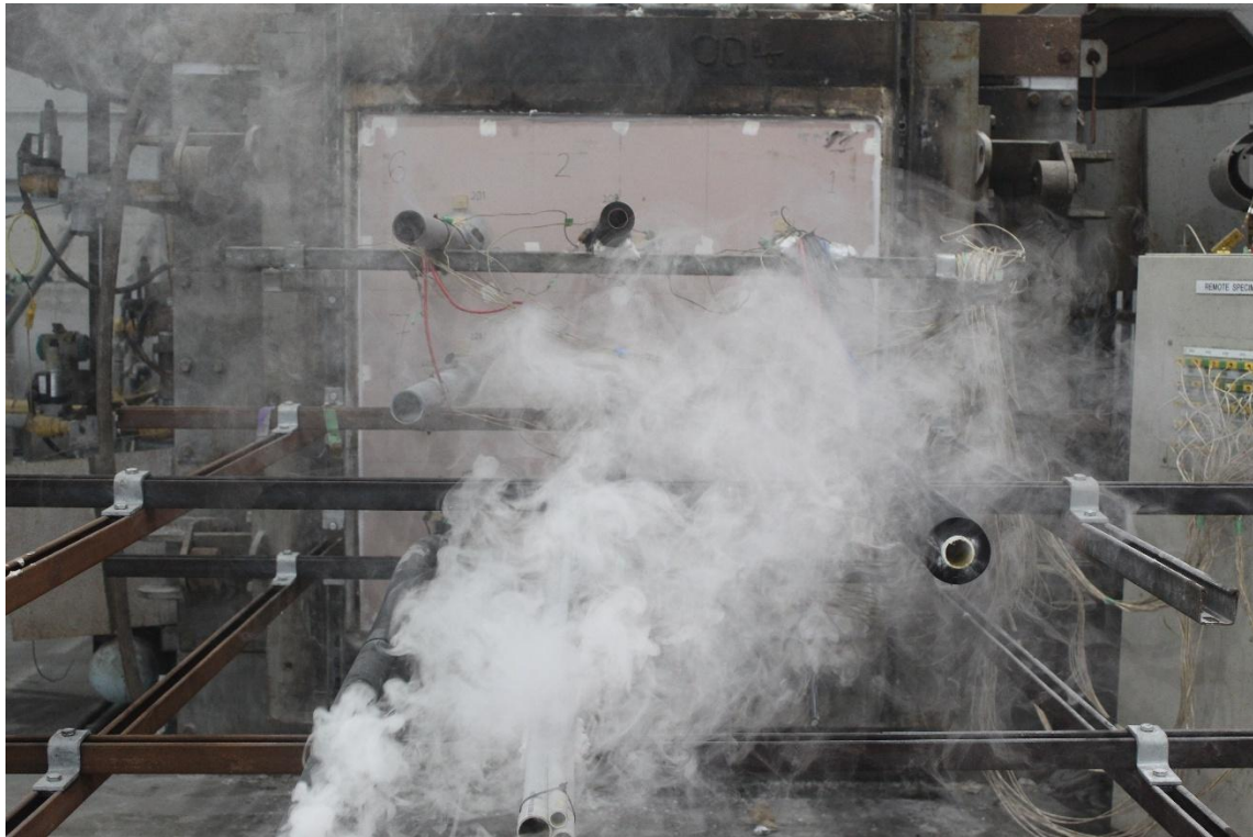
Figure 26 - Unexposed face at 15 minutes
