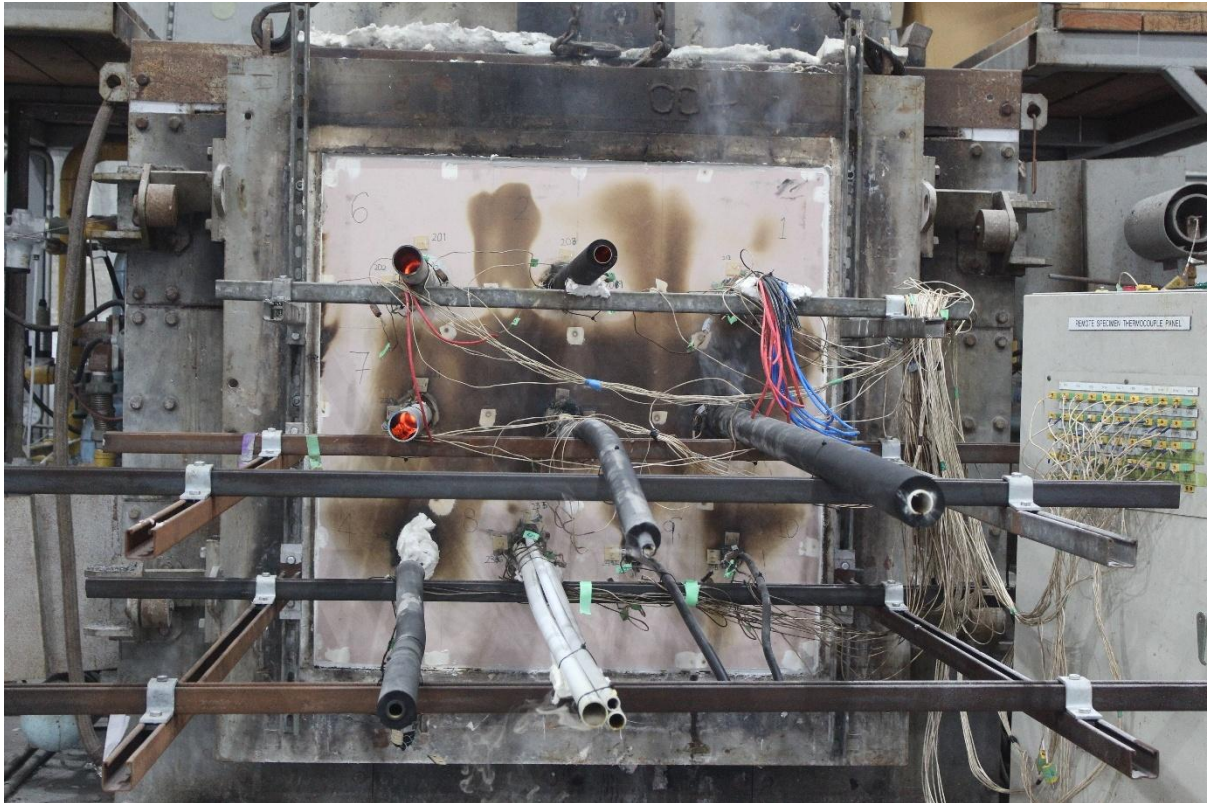
Figure 34 - Unexposed face at 90 minutes
