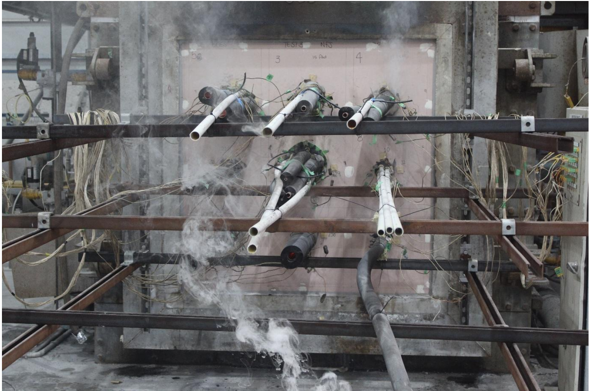
Figure 28 - Unexposed face at 45 minutes
