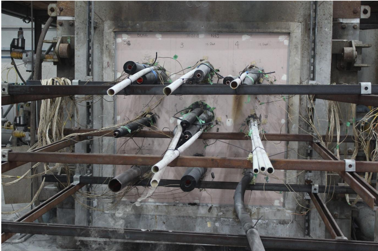
Figure 32 - Unexposed face at at 75 minutes
