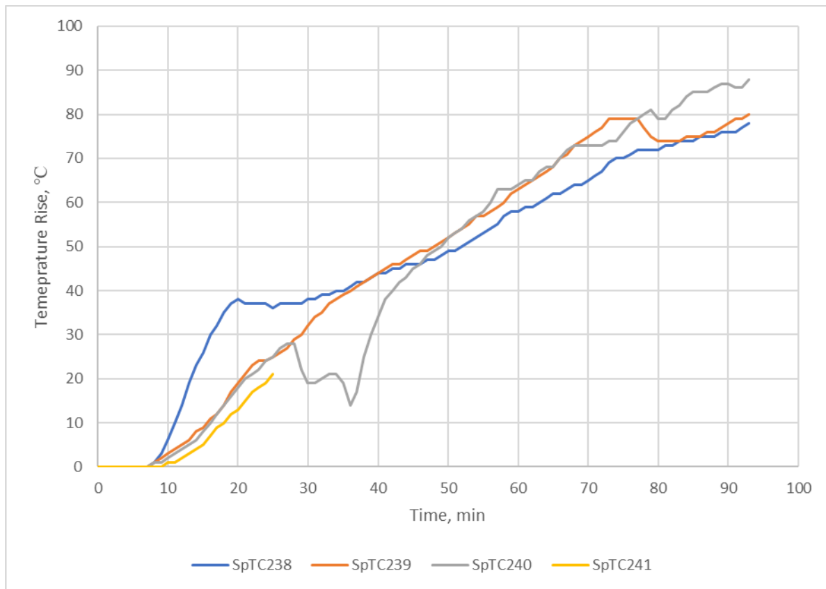
Figure 21 - Specimen 9 thermocouple temperature rise readings
