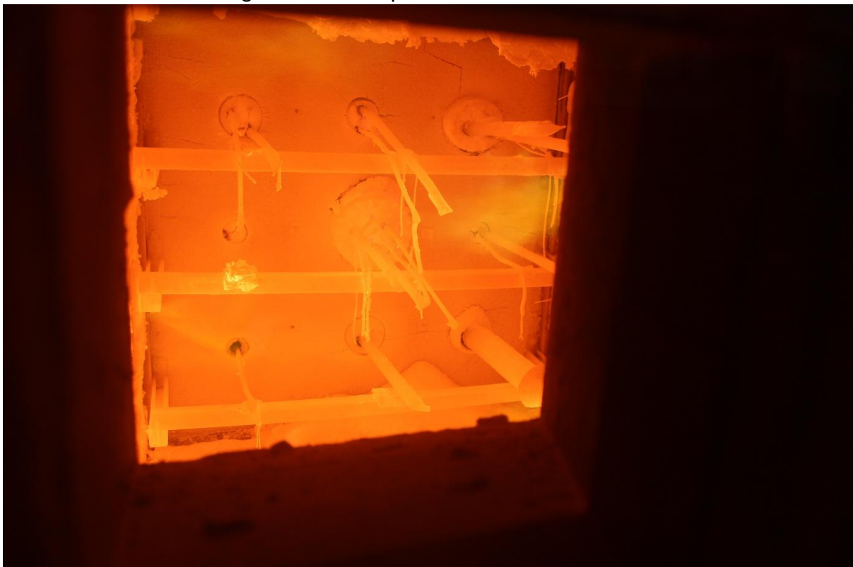
Figure 33 - Exposed face at 75 minutes
