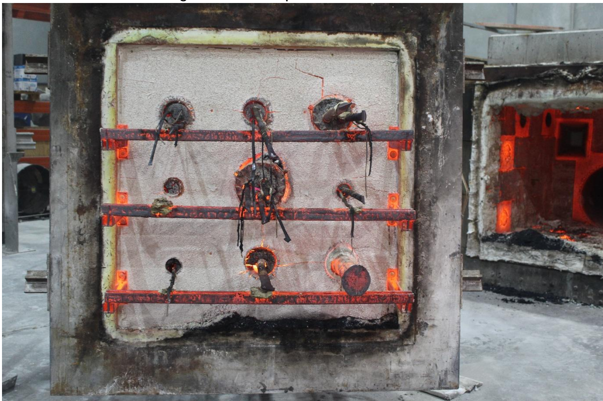
Figure 35 - Exposed face after the test
