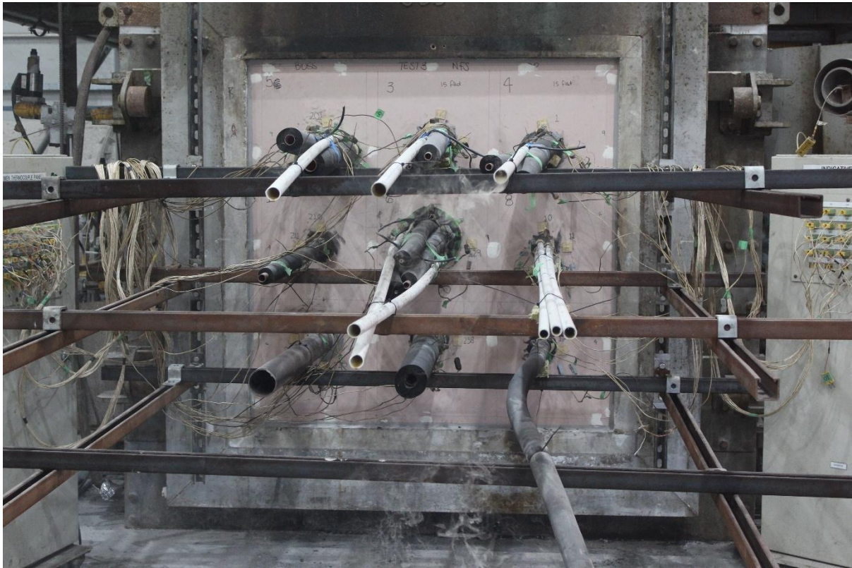
Figure 24 - Unexposed face at 15 minutes
