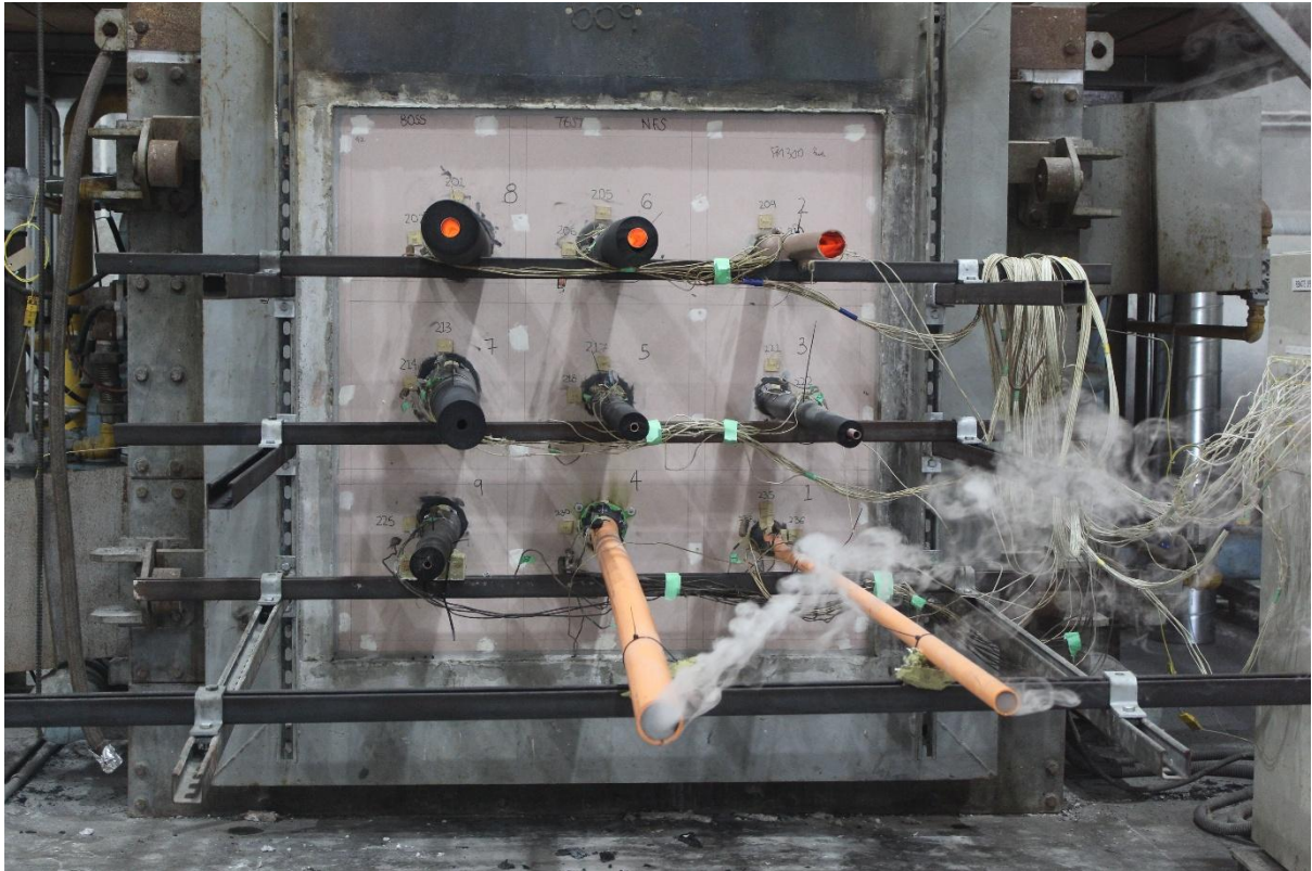
Figure 30 - Unexposed face at 60 minutes
