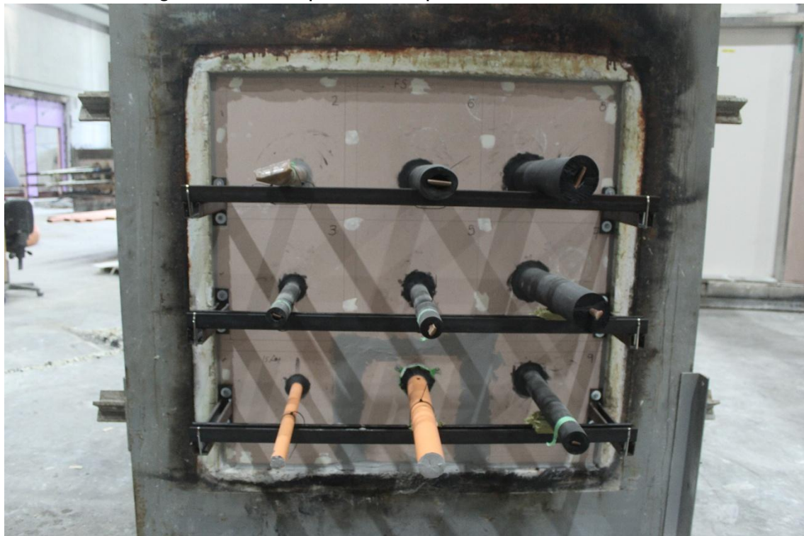
Figure 23 - Exposed face prior to test commencement
