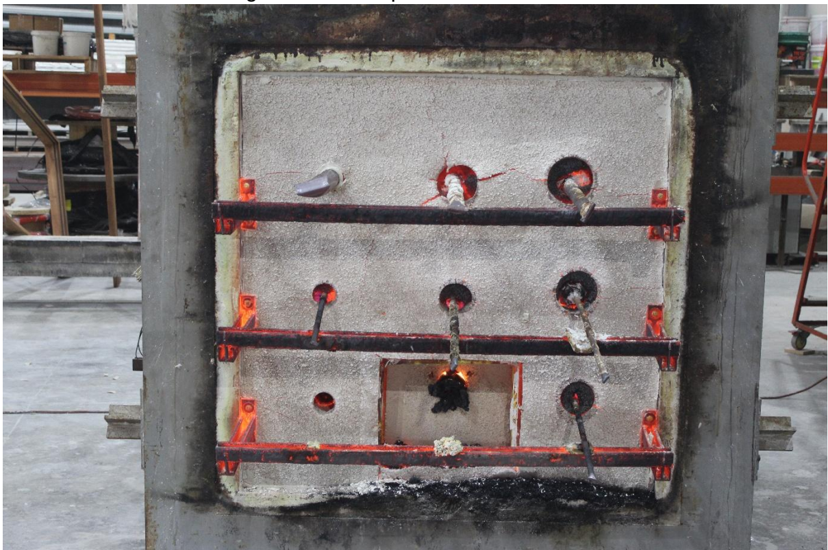
Figure 35 - Exposed face after the test
