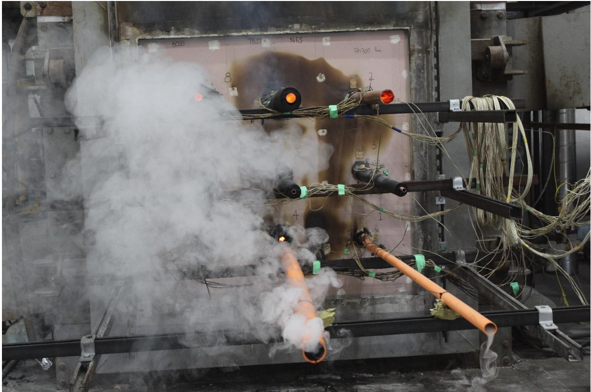
Figure 34 - Unexposed face at 90 minutes
