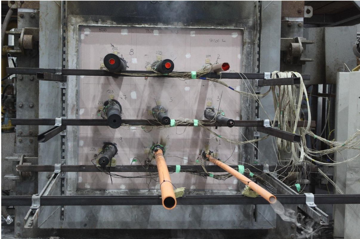
Figure 26 - Unexposed face at 30 minutes
