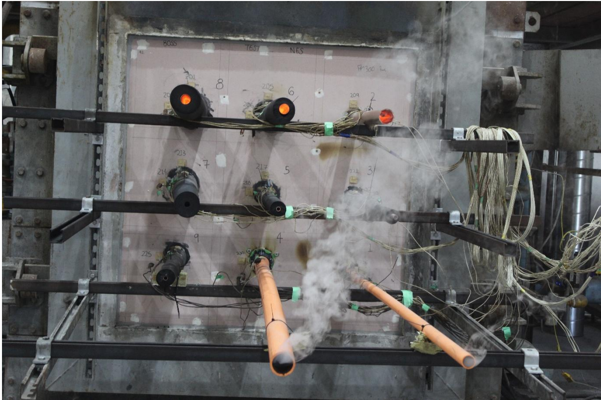
Figure 32 - Unexposed face at 75 minutes
