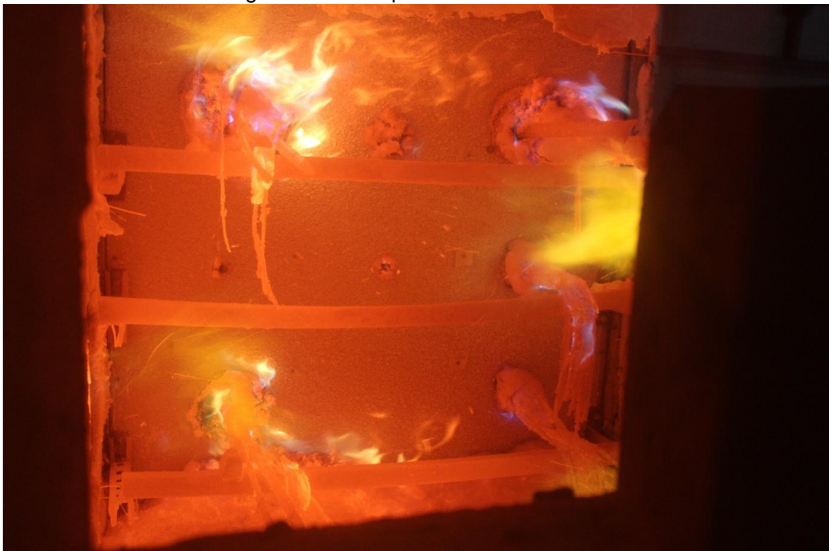
Figure 27 - Exposed face at 30 minutes
