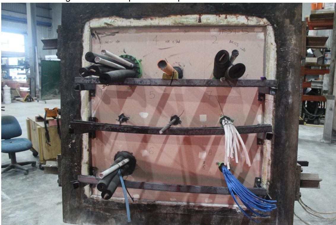
Figure 23 - Exposed face prior to test commencement
