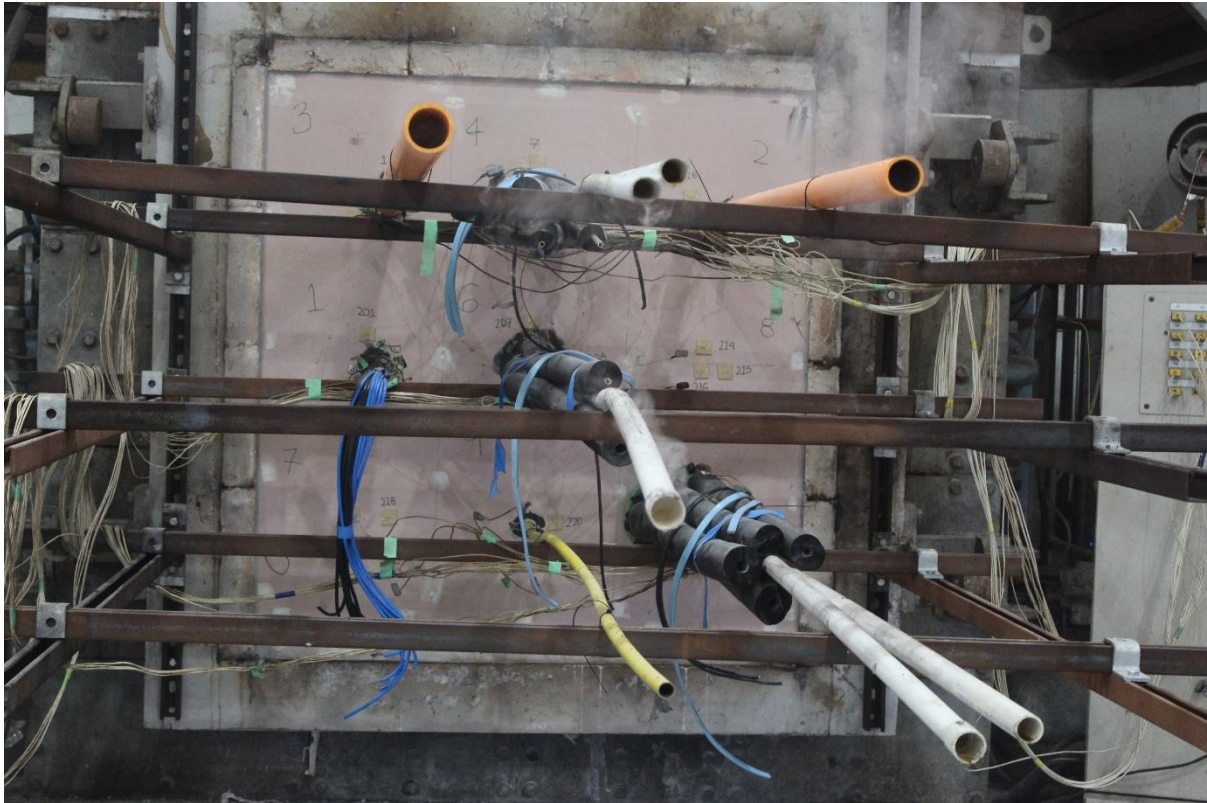
Figure 26 - Unexposed face at 30 minutes
