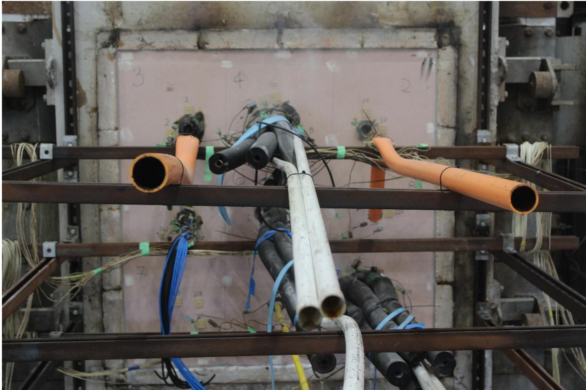
Figure 34 - Unexposed face at 120 minutes
