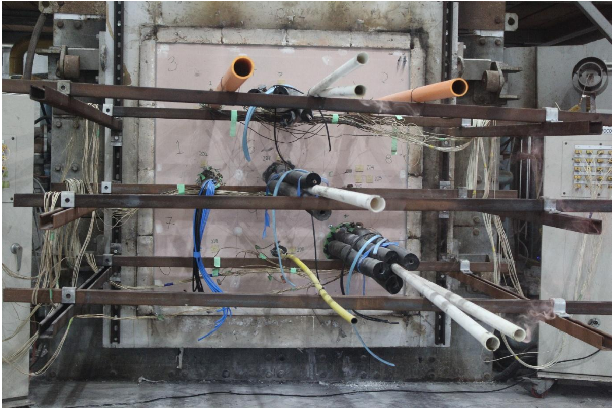
Figure 24 - Unexposed face at 15 minutes
