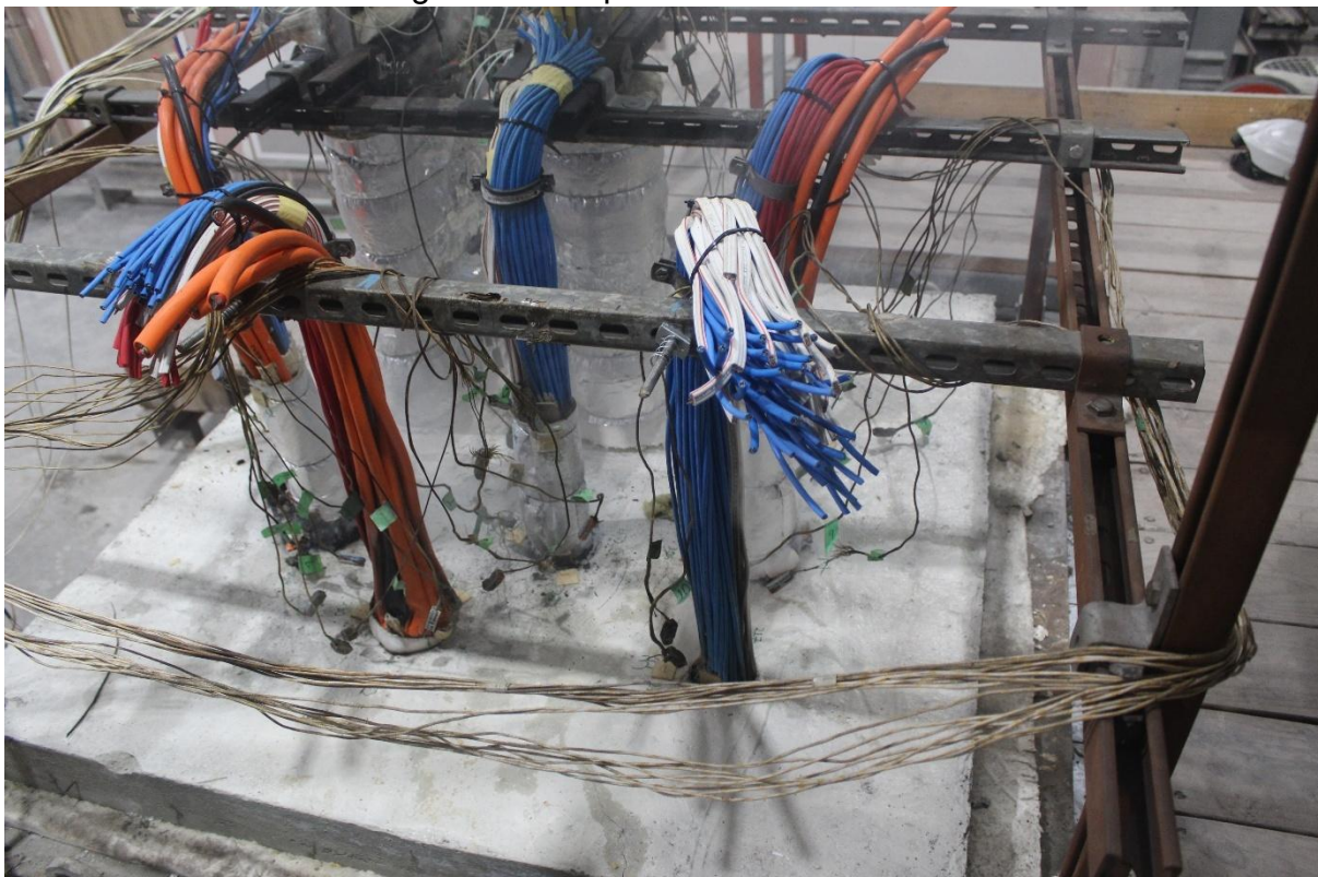
Figure 33 - Unexposed face at 90 minutes
