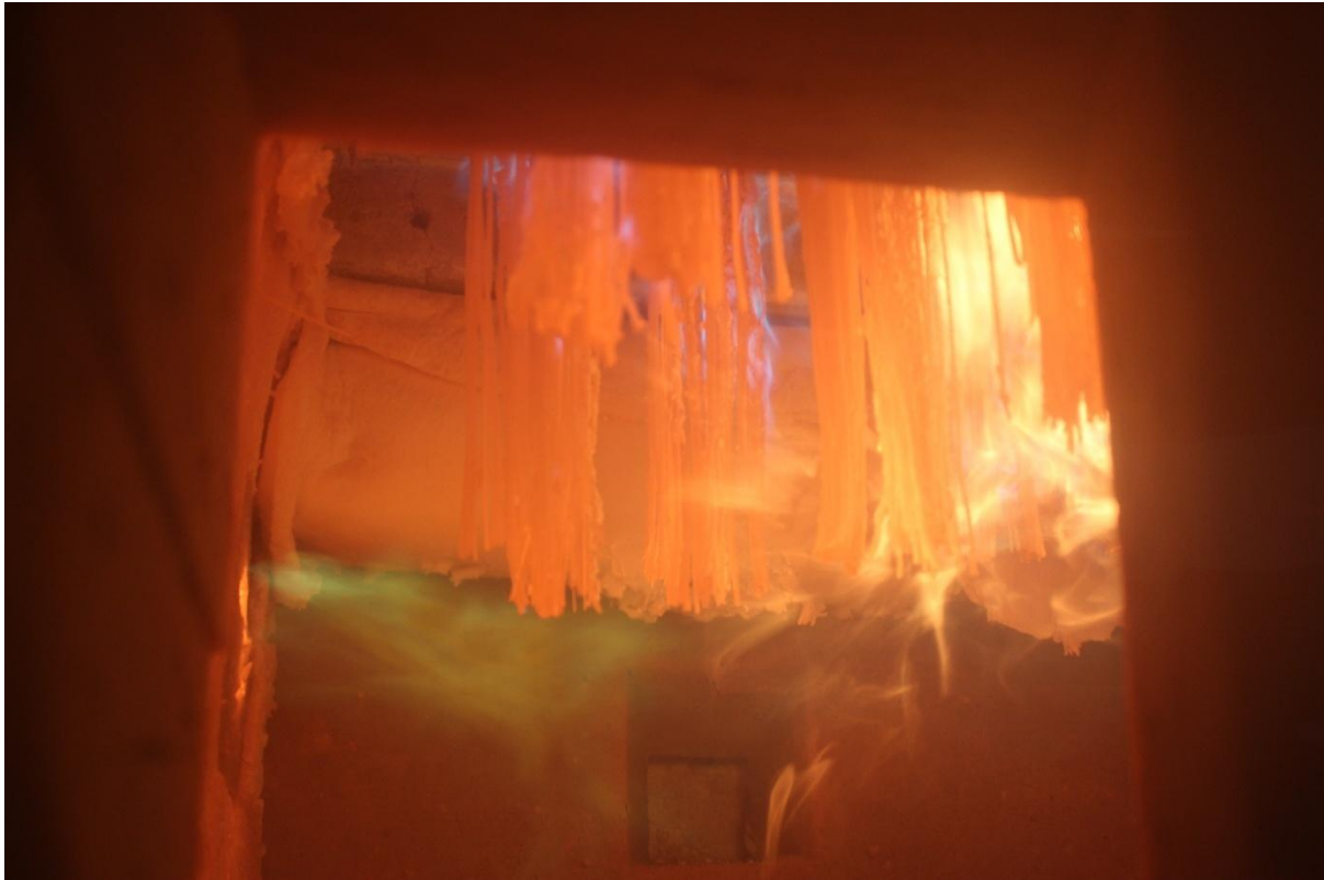
Figure 30 - Exposed face at 45 minutes
