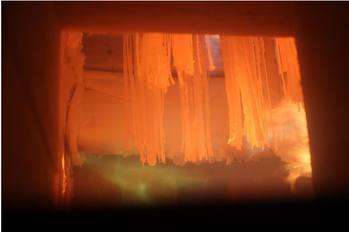
Figure 32 - Exposed face at 60 minutes
